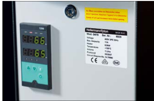
Professional type plate on a heating unit.
