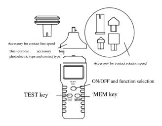
Attention: Photoelectric type measurement is recommended during measurement of high rotation speed for sake of safety.
